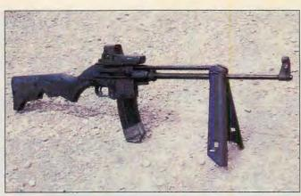
If desired, the SU-16's fore-end quickly unlocks to become a bipod. (below) Kel-Tec's SU-16 is shown in OD green and desert tan, and the new SU-16B is seen with a black stock.
